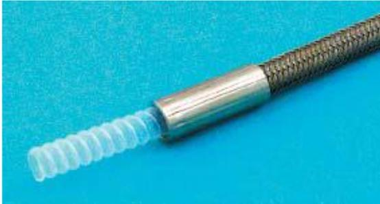
We recommend PTFE when you want a high durability and the application demands high chemical resistance. The hose is designed with an corrugated inner tube from PTFE and an outer braid in stainless steel (for standard AISI 304) is used. We also produce high performance hoses with innertubes in other fluoroplastic materials such as PFA, ETFE and PVDF or with a covering from Hytrel®.
